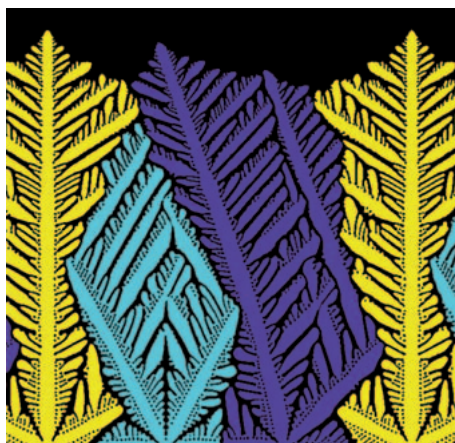
Fig. 4. Directional growth of a ternary Mg-alloy (Al-Zn-Mg). Simulation made with MICRESS®. Note the hexagonal symmetry of the dendrites. Picture size corresponds to an area of approximately 1*1 mm 2 .
